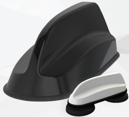
The MiMo Sharkee range offers 2x2 MiMo 698-960/1710-3800MHz with active GPS/GLONASS (26dB LNA) and optional SiSo or 3x3 MiMo WiFi 2.4/5.0GHz. With a built in whip mounting boss the MiMo Sharkee can also support a range of Panorama Antennas' VHF/ UHF whips (Except SHKG-7-27-T24-58).
